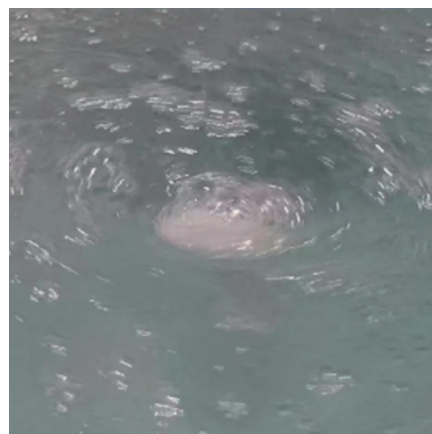
105rpm Liquid level 2000L(full load) Top bubble distribution
